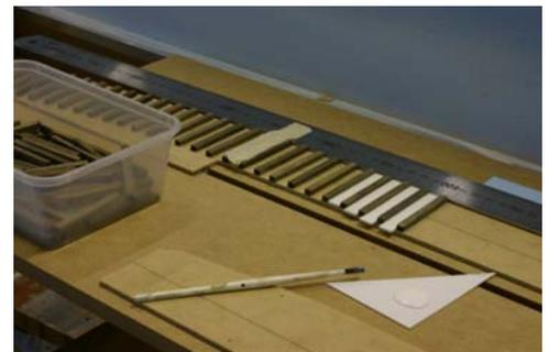
Once my sleepers are dry and ready to lay, I set out a datum line on the section of the layout using the edge of a steel straight edge – of course this is only applicable for straight track. I like to use a centre line for track laying rather than relying on the edge of the sleepers as a guide because some of them are longer than others. I paint the back of the first sleeper with a
