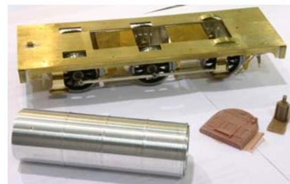
*18 Class Components – This photo shows the progress with some of the Berg's 18-class project components. The boiler turning was hot off the presses and will be cast in urethane. Also pictured is the backhead that will be supplied with the kit.*
