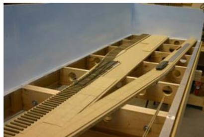
*In this photo (which is a different point to some of the earlier photos), you can see where I've installed the 3mm MDF insert with the point in place and have laid some more sleepers up to the edges of the point. I'll lay rail on the plain track starting from the point and working outwards. The sleepers are laid using PVA.*
