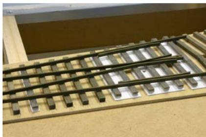
*This picture shows the frog in place and painted and you can clearly see the feeder wire soldered to the side of the casting. You can also see the way I've packed out the copper clad sleepers with styrene. I don't bother fiddling about with thin strips but just shove in a large sheet. The whole thing will be covered in ballast eventually so none of this will show.*
